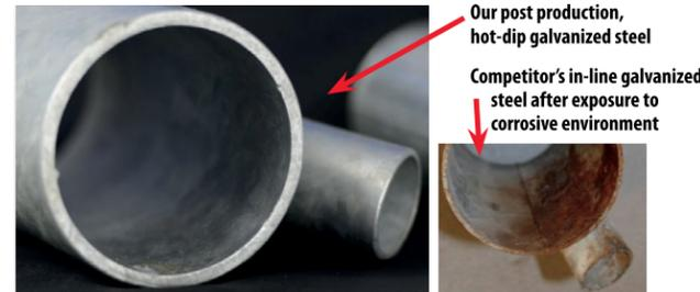
Salt is highly corrosive and can compromise the integrity of steel components. Our frames and welded components receive a hot-dipped galvanized finish *after* fabrication to ensure a complete zinc coating both inside and out. No welding is done after zinc coating is applied. Some competitors cut corners and do not hot-dip galvanized welded components.
