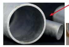
Our post production, hot-dip galvanized steel Competitor's in-line galvanized steel after exposure to corrosive environment
